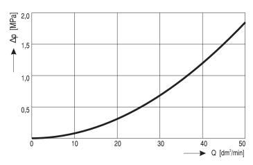
Characteristic of the check valve  $\Delta p$  = f(Q) M 06-4 M 06-A-4 M 06-B-4
