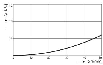
Characteristic of the check valve  $\Delta p$  = f(Q) M 10-4
