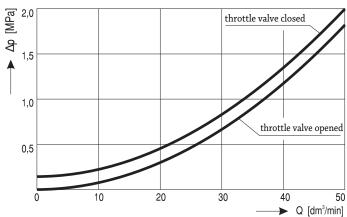
Characteristic of the throttle valve  $\Delta p$  = f(Q) M 10-4
